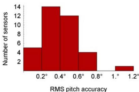
Fig. 2. Distribution of pitch accuracy over sensor sample
