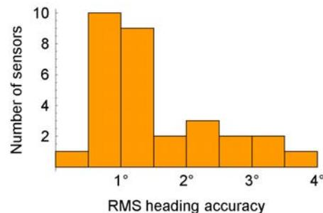
Fig. 3. Distribution of heading accuracy over sensor sample
